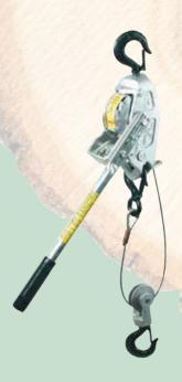
These Lug-All pullers offer many features that make using cable pullers easy. Each one has a high strength alum alloy frame and an interlocking pawl system. All cable stores on a drum. Along with the self-cleaning open construction and reversible safety handle, it has oiled for life bearings. It uses forged steel safety hooks. An extra hook and pulley are included. It has self-cleaning open construction for its highly flexible 7 x 19 Aircraft Cable. It comes in a variety of sizes.
