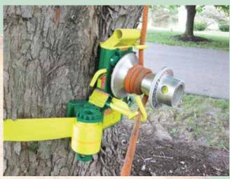
Key arborist tool since 1980, this heavy-duty ratcheting bollard allows for excellent control while rigging. Hourglass-shaped drum keeps rope centered while lowering. Utilizes trucker bar to pull tension on drum and strap. Bar and strap included. Shipping Wt. 66 lbs.
