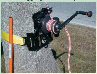
Designed and tested by arborists, the GRCS is the most advanced tensioning and lowering bollard available. The tensioning winch is a double geared, roller bearing, two-speed winch having a 44:1 high power slow speed gear and a 22:1 lower power high speed gear. Best of all, the winch is self-tailing. No one needs to keep tension on the bull rope. The GRCS also comes with a fixed bollard post for those times when tensioning the bull rope is not critical. Shipping Wt. 90 lbs.
