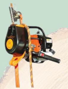
Motorized ascender. Pulls climber to the top of large trees effort-lessly at up to 100 feet per minute travel speed. Built-in failsafe systems and integrated emergency retreat system. The compact two-stroke gasoline enging has a powerful gear reducation system producing lift capacity of 300 lbs.
