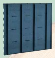
DeepRoot Universal barriers are an ideal solution for tree planting in areas proximate to hardscaping or structures. Barrier panels are 2 foot long panels available in heights of 18", 24", or 36". Panels flex to allow for linear or surround installations. Panels are made of recycled plastic with UV inhibitors for long product life. For most tree planting applications, UB18-2 and UB 24-2 are the barriers of choice.
