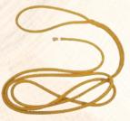
14' or 12' load balancing rigging sling of Tenex with 12' eye splice in one end. Use 3/8" size on 1/2" bull rope and 1/2" size on 5/8" bull rope. Shipping Wt. 3 lbs. each
